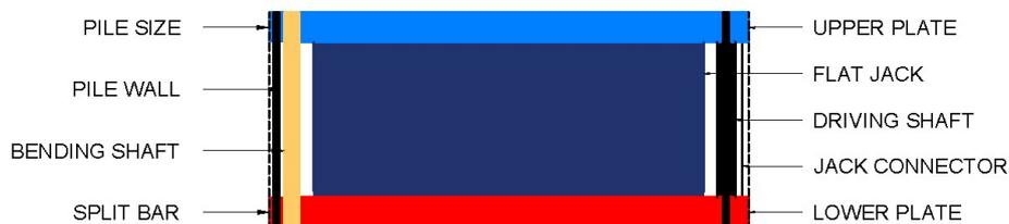
OJACK360 is a hardware system to measure load-displacement of a pile when loaded in bi-directional static axial compressive loads with using an embedded bi-directional jack assembly. The keyword of 360 is comprehensive jack system to be applied on cast bored pile and precast concrete piles.
